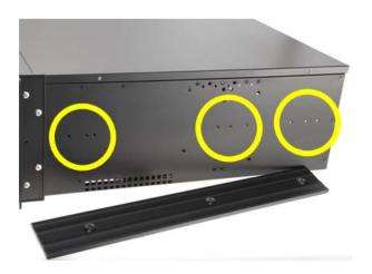
**3.** Upon removing the side bar, you will find several screw holes for you to install the server rail.
